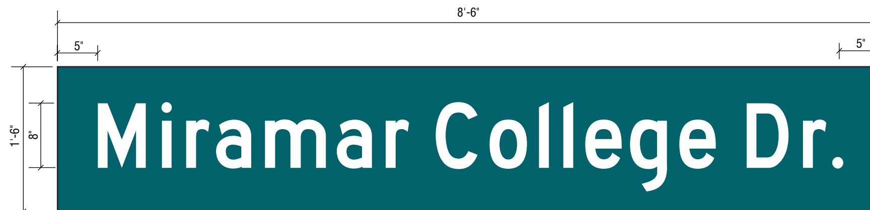
FRONT VIEW - STREET NAME PLAQUE FOR MAST ARM SCALE: 1' = 1'-0"
