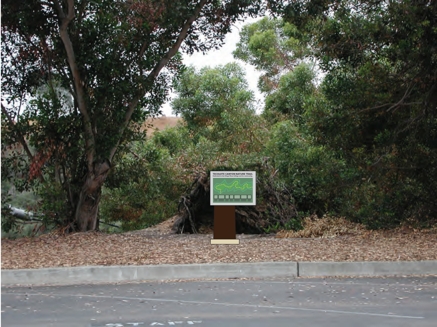
INTERPRETIVE SIGN AT ENTRY TO TECOLOTE CANYON TRAIL. INFORMATION PANEL MADE OF HIGH-PRESSURE LAMINATE MATERIAL. PEDESTAL MADE OF CORTEN STEEL ON A STAINED CONCRETE PAD.
